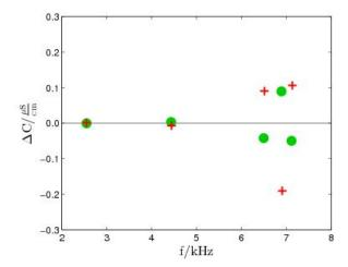
Difference between calibration measurements and a cubic fit ('residual error') for two independent calibrations. Green dots for results of 29.4.2015, red crosses for those of 3.4.2015.
